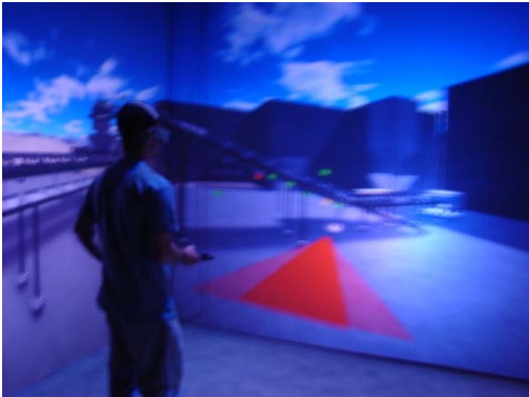
Figure 5. The CAVE version of the instructional tour virtual environment for conveyor systems
