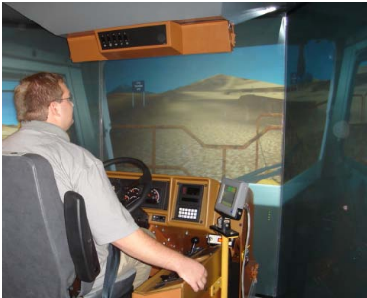
Figure 1. An example of a simulator used for training haul truck operation
