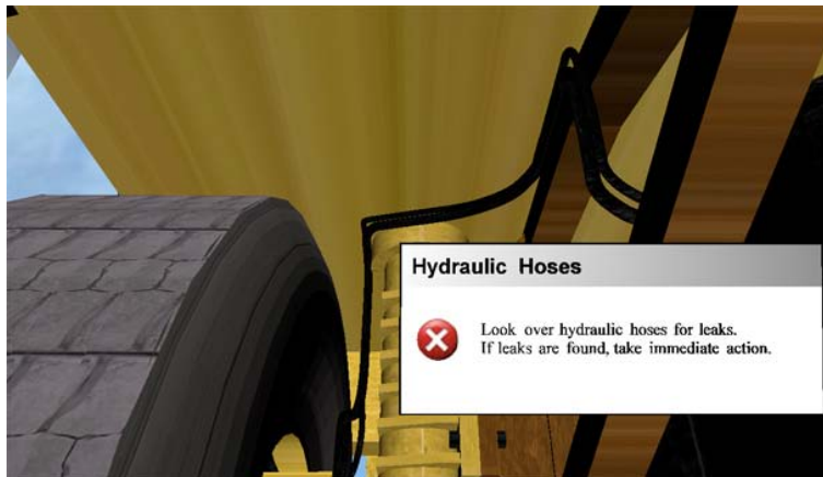
Figure 2. Example hydraulic hose inspection point and associated information window
